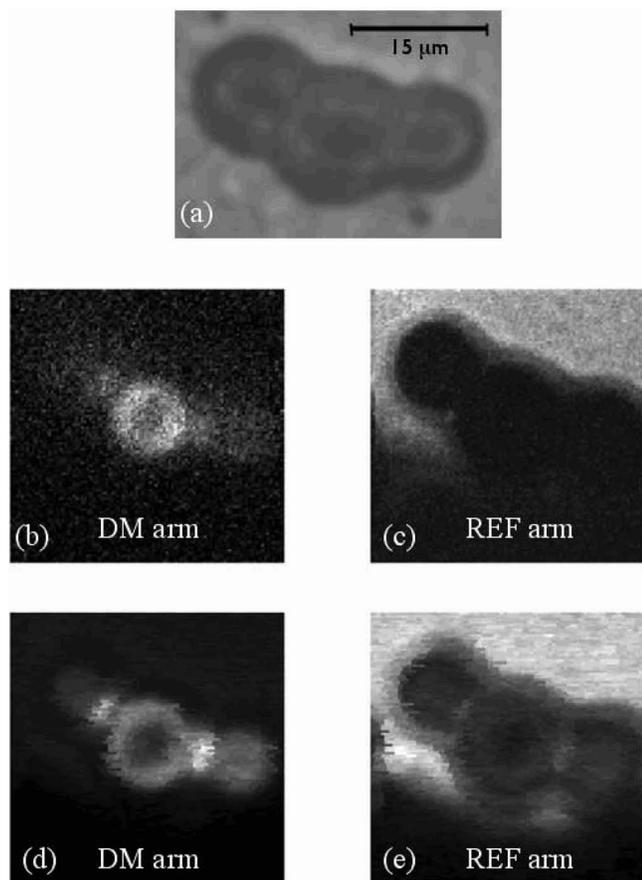
Fig. 3. Images of  $15\ \mu\text{m}$  microspheres on Lucifer yellow dye and suspended in agarose: (a) white-light microphotograph of the scanned area, (b) and (c) TPA fluorescence images obtained by blocking the delay (DM) arm of the microscope and using conventional acquisition scheme, (d) and (e) TPA fluorescence images obtained simultaneously using the SMARTI technique. All TPA images are  $101 \times 101$  pixels REF, images from the delayed arm.
